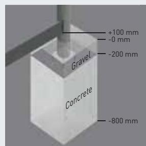
Pre-drill the holes on the post for the base plate (75 x 850 mm). Screw the base plate to the oval post (3 M8 x 80). Fasten the base plate complete with post to the foundation using a suitable anchoring system. All posts must be vertically aligned.
