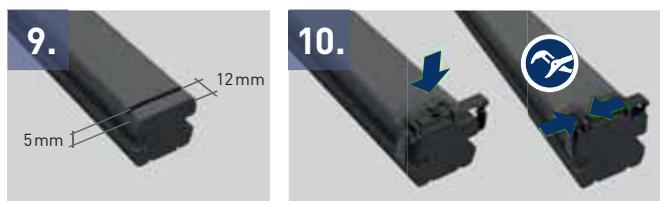
Mounting the closing strips: please refer to items 16 to 18 when assembling with concrete kerbstones
