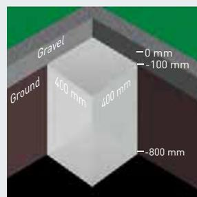
A separate, suitable foundation is required. For this purpose, dig all of the foundation holes (400 x 400 x 800 mm) and fill with concrete to a height of between -800 mm and -200 mm. Allow to fully harden. Alternatively, a suitable anchoring system can be installed on-site.
