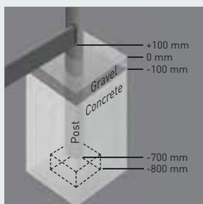
Fill the foundation hole with concrete to a depth of 100 mm. Position the frame in the foundation hole at a depth of -700 mm. Precisely apply the lower edge of the post with the aid of a small brick. Apply concrete into the foundation hole to a level of -100 mm. All posts must be vertically aligned.
