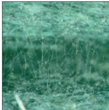
Fig. 7: Mould on test specimen 59 (H40), 40-fold enlargement.
