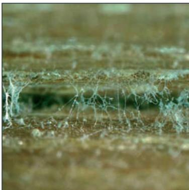
Fig. 9: Mould on test specimen 77 (Bangkirai), 50-fold enlargement.
