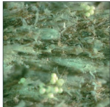
Fig. 8: Mould on test specimen 72 (H41), 70-fold enlargement.
