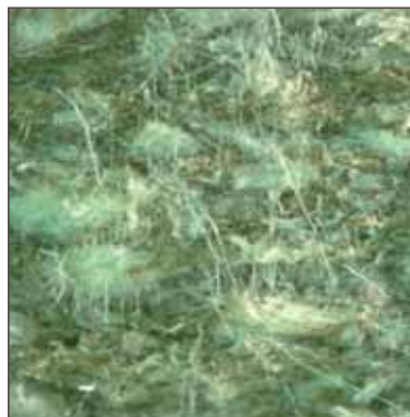
Fig. 10: Mould on test specimen 122 (H41), 40-fold enlargement.
