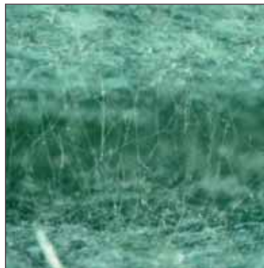
Fig. 7: Mould on test specimen 59 (H40), 40-fold enlargement.
