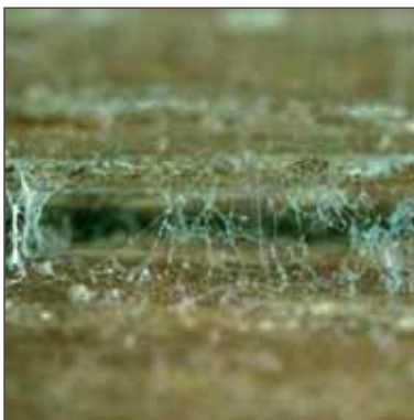
Fig. 9: Mould on test specimen 77 (Bangkirai), 50-fold enlargement.
